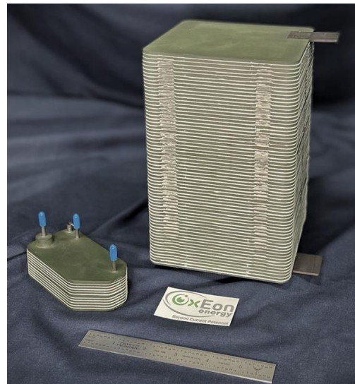
Figure 1. Size comparison between MOXIE SOXE and mission-scale SOXE stacks.
